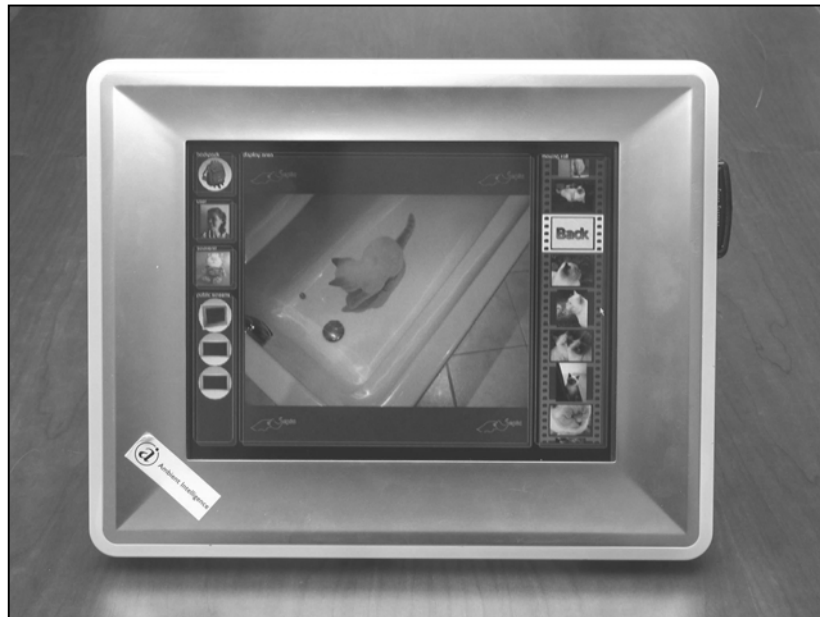
Fig. 5.6. The third and final version of the Digital-Photo-Browser user interface and device, with LED's in the casing (white rim bordering the device). As can be seen in the left part of the UI, the cat-object is active (the third picture from the top) and the roll contains the photos associated with this object. (For the explanation of the back-pack picture in the top-left corner of the user interface, see Qian, 2004.)
