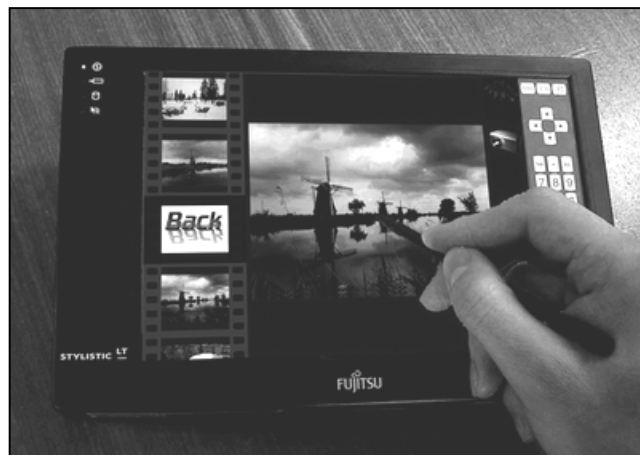
Fig. 5.4. The first version of the implemented Digital Photo-Browser user interface and device.
