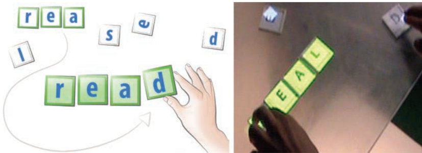
Fig. 6. Connecting Cards (left side: scenario; right side: implementation) can be used to create words with letter cards and get feedback about whether the word is correctly spelled or not.
