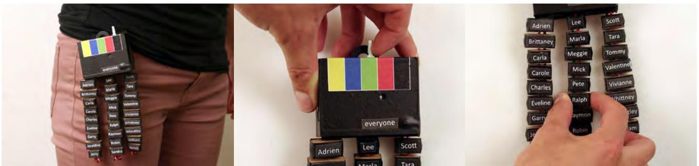
**Figure 2. FireFlies Teacher-Tool: clipped to the user’s clothes (left), selecting a color (middle) and selecting a child’s name (right).**
