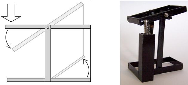
Figure 3. Iconic bridge, schematic (left) and prototype (right).
