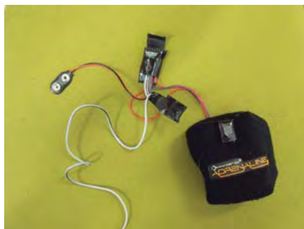
Figure 1: Sensor band for sensing bow length. It is worn near the elbow and uses a gyroscope to measure what angle the elbow moves through as the player bows.
