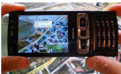
Figure 2. The MapLens prototype, which appends digital information to the camera view of a paper map.
