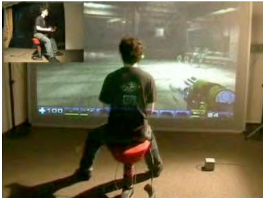
Figure 1. Use of the ChairIO in a first-person shooter game as intuitive navigation method completely controlled by implicit body skills.
