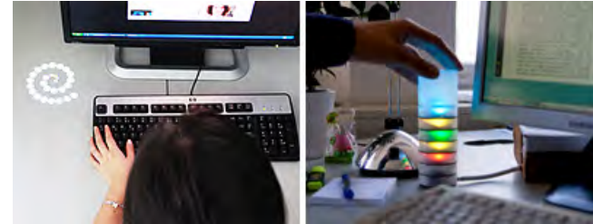
figure 1. Two prototypes: the ambient appointment projection (left) and the tangible presence indication (right)
